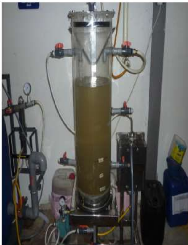
Figure 2: Schematic for Ultrasonic Membrane Anaerobic System (UMAS)
